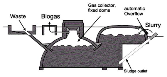
Figure 5: Fixed dome plant CAMARTEC design
