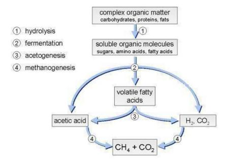
Path of Anaerobic Digestion
