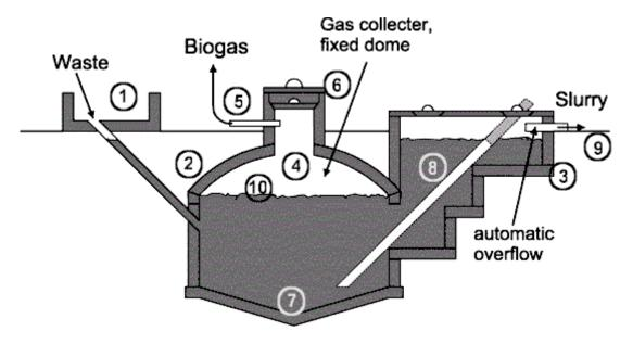
Figure 1: Fixed dome plant Nicarao design: 1. Mixing tank with inlet pipe and sand trap.2. Digester. 3. Compensation and removal tank. 4. Gasholder. 5. Gaspipe. 6. Entry hatch, with gastight seal. 7. Accumulation of thick sludge. 8. Outlet pipe. 9. Reference level. 10. Supernatant scum, broken up by varying level.
