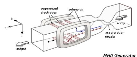
Faraday linear nozzle with segmented electrodes
