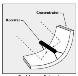
Fig. 1 A parabolic trough
