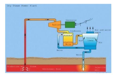
Figure 4: Geothermal Power Plant with Water Cooling System
