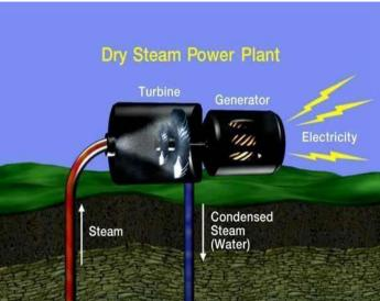
Figure 2: Flash and Dry Steam Power Plant Diagrams
