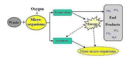
Path of Aerobic Digestion
