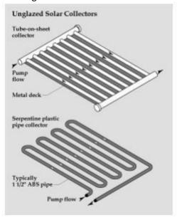
Unglazed solar collectors typically used for swimming pool heating.
