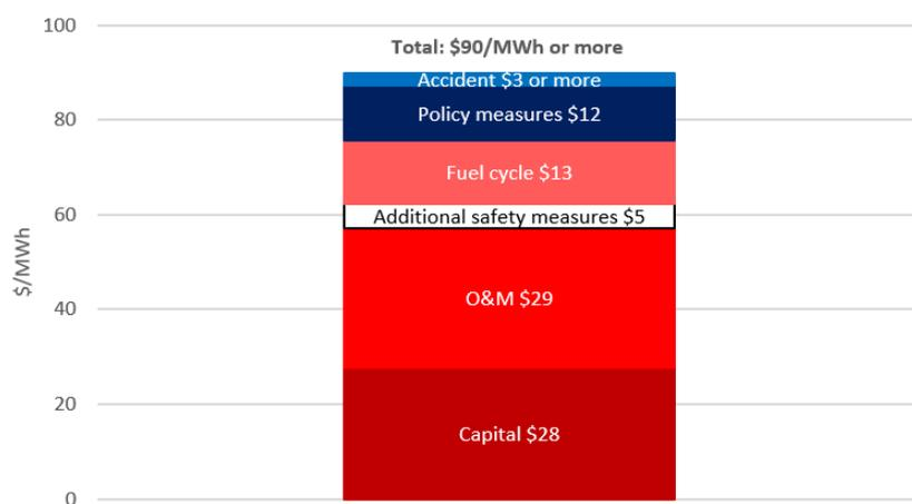
Notes: main assumptions include; installed capacity of 1.2GW, capacity factor of 70%, discount rate of 3%, operation lifetime of 40 years, construction costs of about \$3,300/kW, decommissioning costs of about \$640 million, and costs of Fukushima Daiichi nuclear accident at about \$110 billion acknowledging these may increase in the future hence the mention “or more” (these latter costs have been re-estimated to approximately \$190 billion in 2016)
