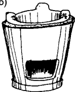
Figure 11.4 Improved efficiency cooking stoves. (a) A large stove designed by the Fiji Ministry of Energy. It is a modification of the Indian (Hyderabad) chula , and is constructed mainly from concrete mouldings. Its operation is described in the text. (b) The 'Thai bucket' stove (sketch). (c) Vertical section through same (units millimetres).
