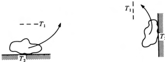
Figure 3.3 Fluid movement by free convection, away from the hotter surface ( T_2 > T_1 ).
