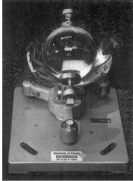
FIGURE 2.31 Campbell–Stokes sunshine recorder.
