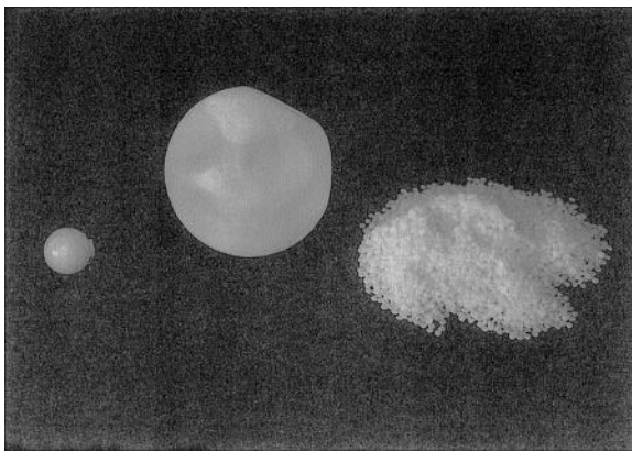
FIGURE 4.2 Examples of commercially developed PCM capsules.
