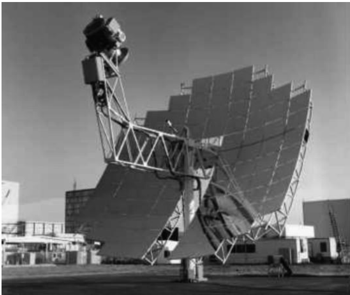
FIGURE 8.31 A 25-kW e dish Stirling system by Stirling Energy Systems, Inc., USA.
